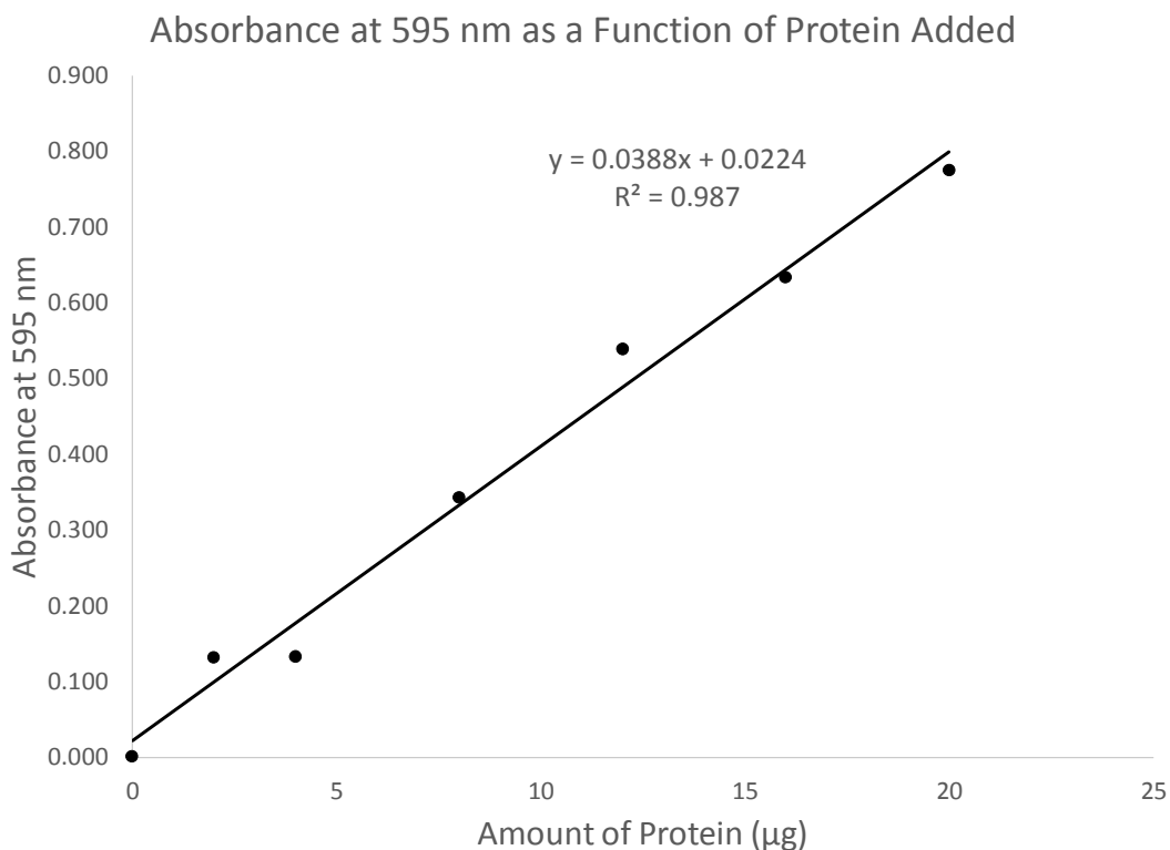
Figure 12. Standard protein curve for protein concentration determination.
